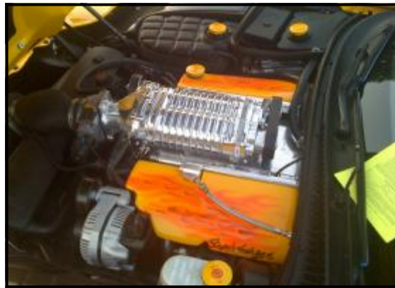
The Magnusson Supercharger produces 535 HP at the wheels while providing 30 MPG at 75 MPH. It is streetable even in heavy traffic.
